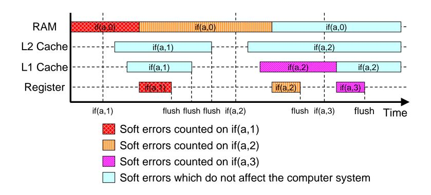
Our estimation technique calculates the temporal and spatial use of every data item at each level of memory hierarchy so that we can calculate the number of SEUs on the data time.
